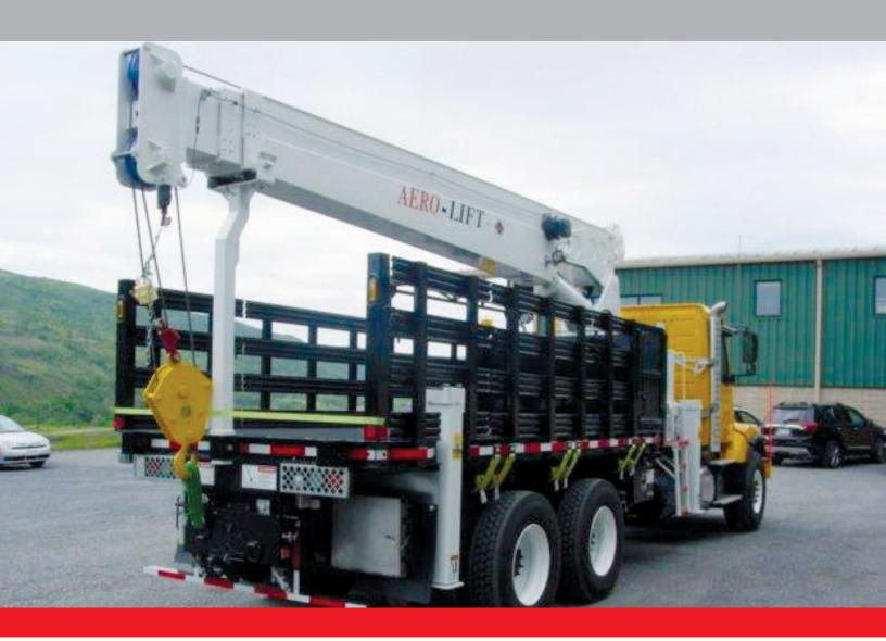
A fully-hydraulic telescopic crane with two boom extensions, LMI load system, and proportional controls. **Simple design that helps elevate your bottom line.**
